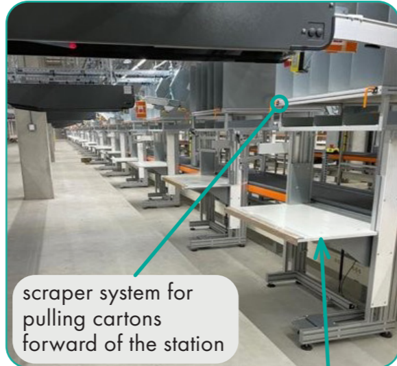
Height adjustable worktop (through a gas cylinder with guide): allows to adapt the height of the table in relation to the height of the boxes, by a simply pushing your hand on the table
