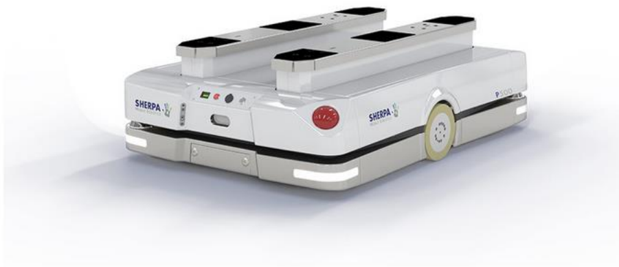
The Sherpa P (Pallet) robot (image courtesy of Sherpa Robotics)
