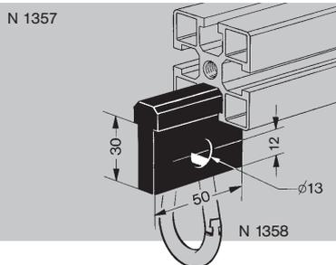
**Guide profile - N 1357** : To hang objects, for example electric or pneumatic tools on a workstation.
