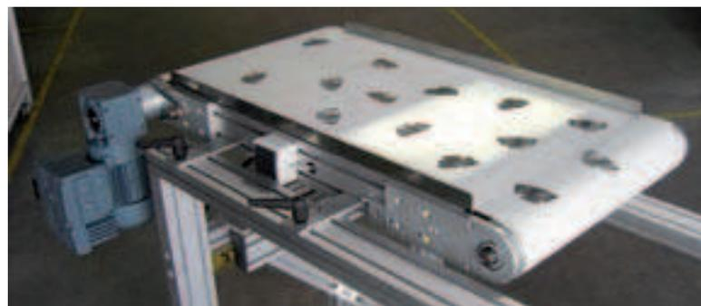
Conveyor with integrated light table for optical identification of sheet steel parts.
