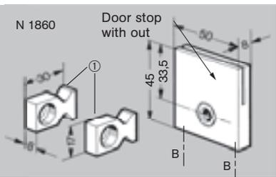
**Kit 1 for quick removal of panels - N 1860** With screws and nuts. For access panels on housings. The panel can be fitted and removed with a single captive screw. To avoid their rotation, the parts ① should always rest on a profile, hinge, etc. otherwise see N 1859 p. 51.
