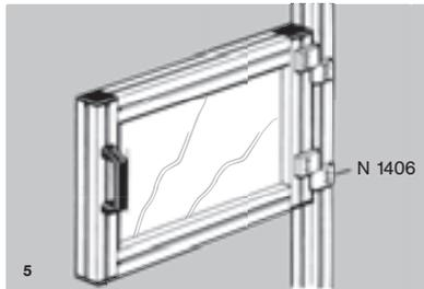
**Doors and windows** of moderate size (up to about 0,2 m<sup>2</sup>, not subject to vibration) can be completely fabricated in organic glass or transparent plastic (acrylic "Plexi", PVC, polycarbonat, PS, etc., fig 1).
