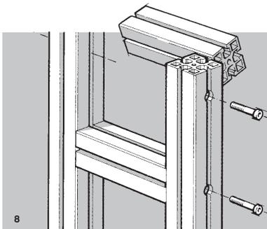
**5.** The M8 tapings in the profile ends are obtained by deformation with a fluteless tap providing increased mechanical resistance (fig. 9).
