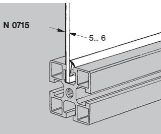
**Mounting strip for 2..5 mm panes - N 0715**: to hold plates and glasses 5 to 6 mm thick in position inside the profile slot.
