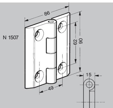
**Hinge 90/49 – N 1507** : with 4 M8 x 20 screws and 4 nuts M8SC. Compatible with "Hiinge kit with switch - N 1509". Maximum opening angle 180°. Material: anodised aluminium alloy.
