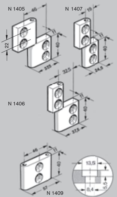
**Hinges** with 4 M8 x 20 screws and M8 SC nuts : consist of two plates in aluminium and one zinc plated steel shaft. The hinges can face left or right and the shaft is locked when assembling. Scale drawing on page 95.
