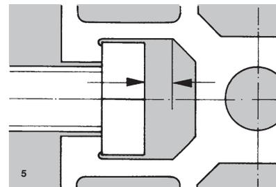
**3.** The M8 SC nuts with **standard M8 square nut dimensions** but with a chamfer can be tilted in the slot (nuts are also available in M6, M5, M4 and M3).
