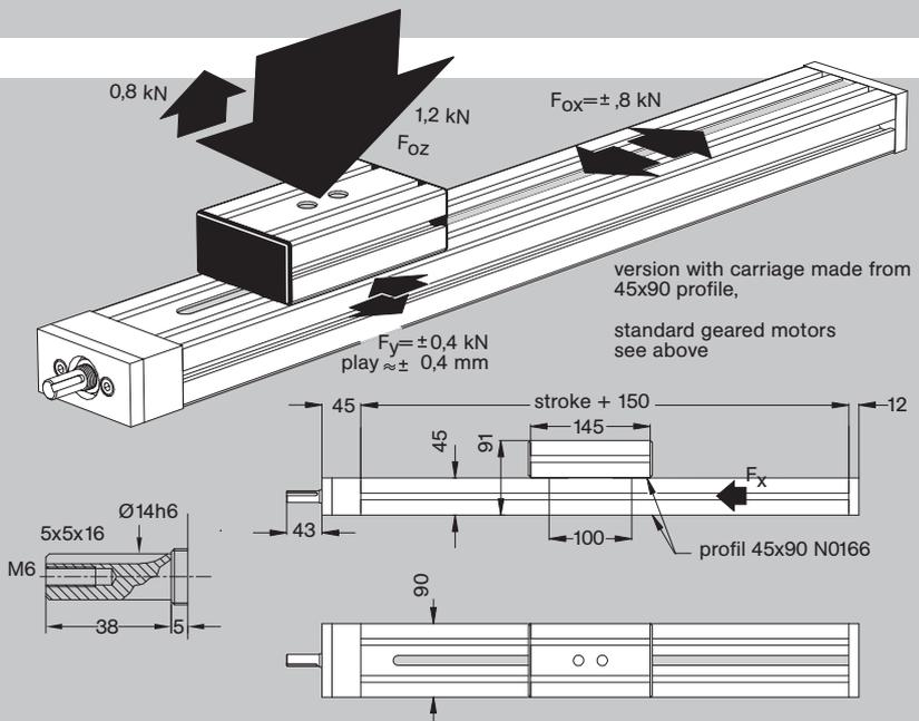
Axial load of the drive screw - the given values incorporate a safety factor of 3 against buckling of the Tr 16x4 screw (pitch:4mm).
