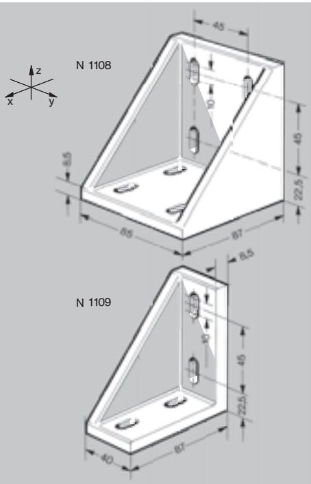
**Corner triangle 87 x 85 - N 1108** : with 8 M8 x 25 screws, washers and M8 SC nuts.
