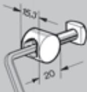
**Assembly nut - N 1140** with M8 x 30 screws and M8 SC nut.
