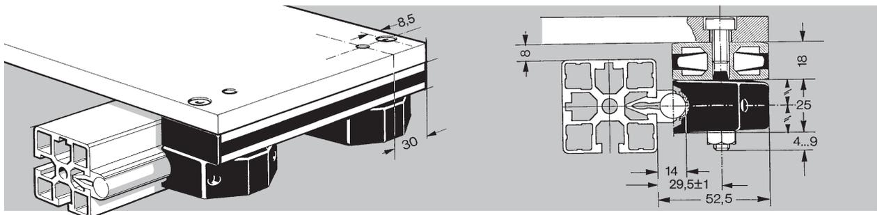
Indirect mountings of K12-cassettes with strut-profile NORCAN 18 x45 mm N 0162. These mountings need cassettes with eccentric shaft N 1930 **on both sides of the rail !**
