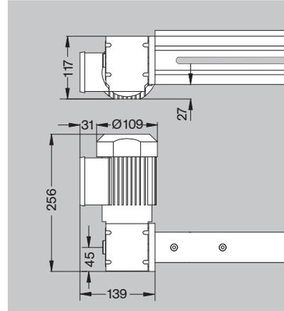
**Linear drive and guidance modules NAPV and K12V** : combination of the linear guide NAP57 (p. 58) or K12 (p. 60) and a trapezoidal screw Tr 16x4 incorporated in a 45x90 NORCAN profile.
