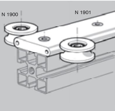
The NAP linear guides consist of an anodised aluminium alloy rail and a 2 or 4 wheeled carriage. Smooth and silent in use, the rollers on shielded ball bearings can be fitted to plates or directly to the NORCAN profiles.
