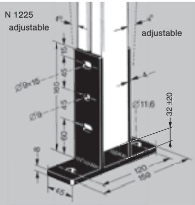
**Anchor Foot 45 x 45 - N 1225** : with 6 screws M8 x 20, washers and M8 SC nuts. For adjustable feet made of NORCAN 45 x 45, 45 x 90 and 45 x 180 profiles. For the last two profiles, two anchor feet may be used.
