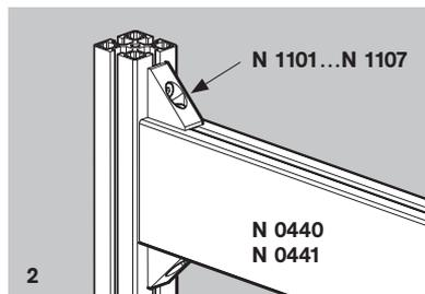
Longitudinal assembly with the assembly nut N1140 (p. 30) or with corner triangles 40x18 N1107, N1103 or N1101 (p. 31).
