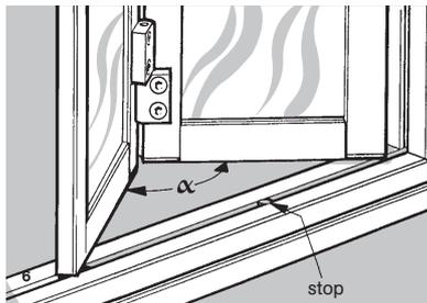
**Folding doors** : Foldings doors are easily made using hinge elements. The angle  $\alpha$  between the two doors must not go below 20° so as to not overload the hinges and pins. (Folding doors supplied ready assembled are fitted with a stop).
