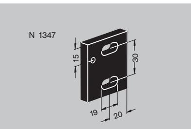
**Guide profile for sliding doors - N1347** : with 2M8x20 screws and 2 washers, for vertical sliding doors framed in NORCAN profiles.
