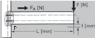
**Method A22** : NORCAN 45 x 90 mm fixed with 2 central screws M8 x 43
