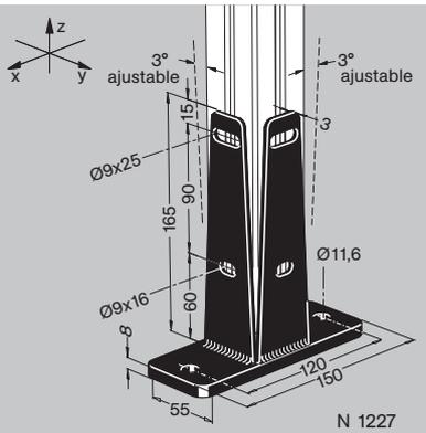
**Anchor foot 45 x 45 half closed - N 1227 :** with 2 M8 x 20 screws, 2 washers and 2 M8SC nuts. Used to anchor uprights made of half closed profiles to the floor.
