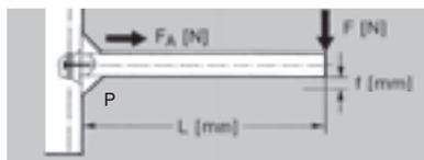
**Method B21 :** NORCAN 45 x 45 mm fixed with a central screw M8 x 43 plus two corner triangles
