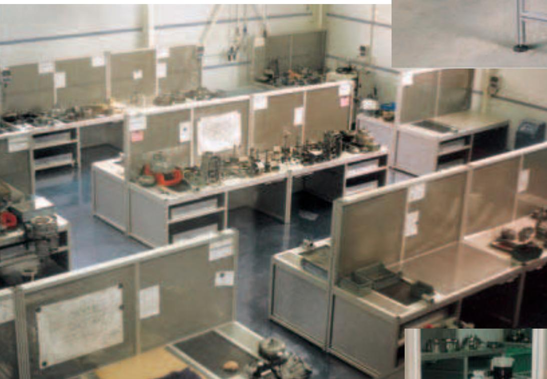
**Above:** Work station for assembling and the computerised inspection of precision guide rails and semi-automatic assembly, inspection and packaging station, with NORCAN frame, housing and conveyor.
