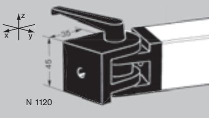
**Pivot 45 x 45 with locking handle - N 1120** with 2 low head screws M8 x 20 mm. Fits on either the cut end or the side of the profile. For fixed angle mountings from +90° to -90°. Maximum torque around the y-axis: 135 Nm (elastic limit).
