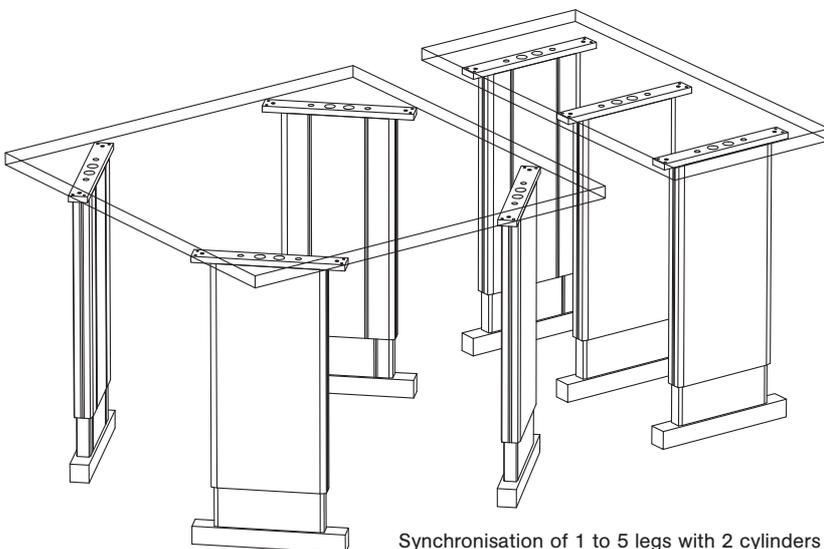
Synchronisation of 1 to 5 legs with 2 cylinders each or 1 to 10 legs with 1 cylinder for adjustable work stations.
