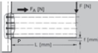
**Method A24** : NORCAN 45 x 180 mm fixed with 4 central screws M8 x 43
