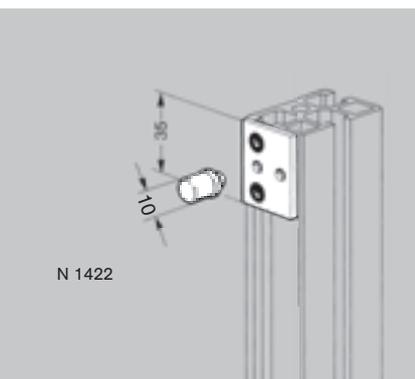
**Ball latch - N 1422** with stainless steel plate and screws and nuts. For doors of moderate size (up to  $\approx$  0,5 m<sup>2</sup>). Two ball latches should be mounted per door in a  $\varnothing$  9,8/12 counterbore, 3 mm deep.
