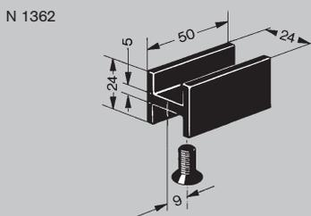
**H-section guide block - N 1362** : with 1 M8 x 16 F screw and 1M8SC nut. For double sliding doors made of 18 x 31,5 mm NORCAN profile sliding on the 45 mm slotted side of any NORCAN profile.
