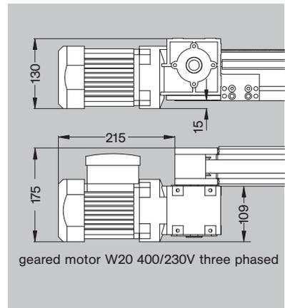
**Linear drive and guidance module K12CC:** combination of the linear guide K12 (p. 60) and a toothed belt AT 5x25 incorporated in a 45x90 NORCAN profile.
