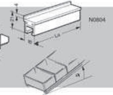
**Slide rail - N 0804** : for gravity feeding small pieces, small containers, circuit boards etc. to workstations. The inclination angle  $\alpha$  must be determined by tests. Material: anodised aluminium, contact face in PE HD.
