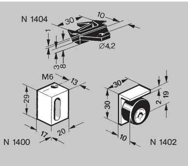
**Panel fixing pad - N 1404** with 4 mm panel screw for mounting panels 19 to 22 mm thick. Maximum static load : 0,5 kN with wood and chip panel, 1kN with aluminium plates.
