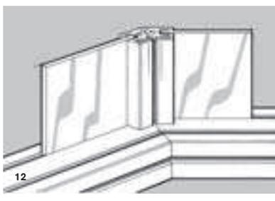
**Angles of 45° (135°) on safety housings :** The NORCAN profile 31,5/45° - N 0195 enables profiles and panels to be joined at an angle of 135° (fig. 11/12).
