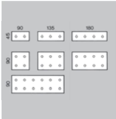
**Assembly plates** with M8 x 20 screws and M8 SC nuts :
