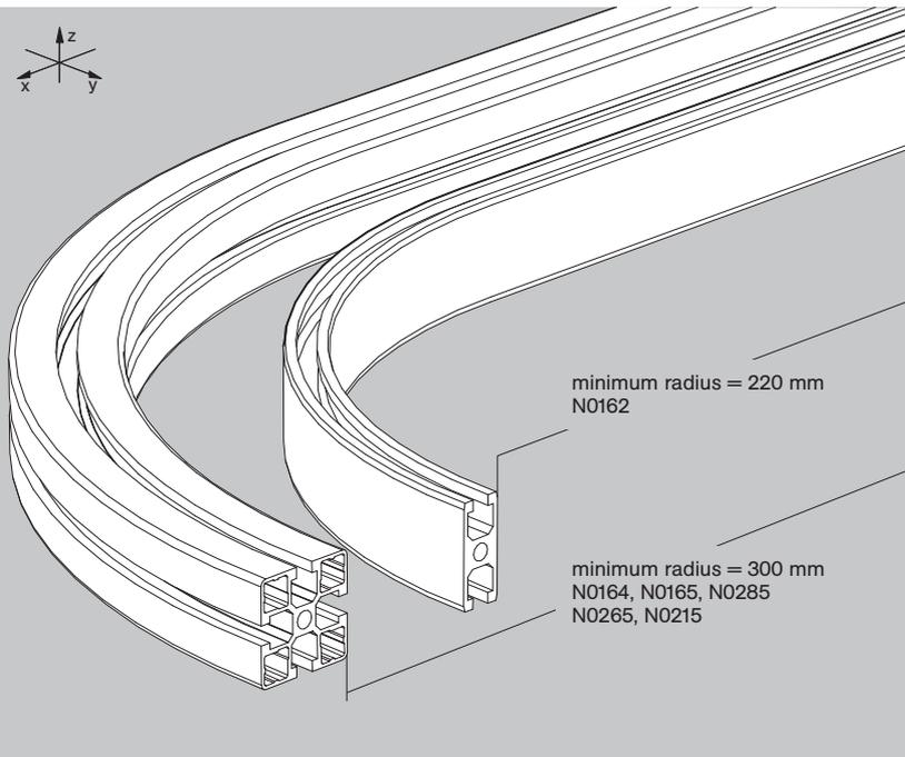
Most NORCAN profiles can be curved. The drawing shows the possibilities for some NORCAN construction profiles.
