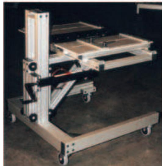
Mobile work station with hydraulic height adjustment horizontal smooth guides and NAP 57 guides with stops.
