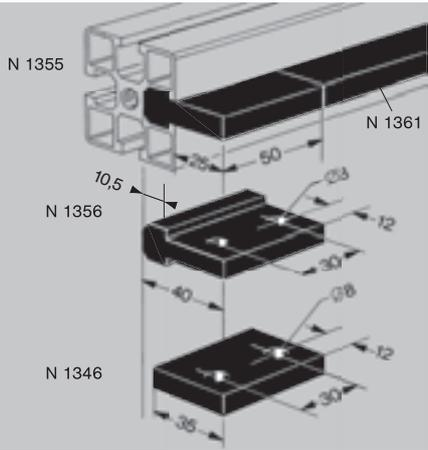
**Guide profiles** in high density polyethylene, black. To make guide rails using the slot in NORCAN profiles.
