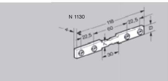
**Angle connection bar - N 1130** with 4 grub screws for end-to-end joints and angle joints under low load.
