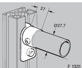
**Joint profile / tube ø27,7 closed - F 1331** with screws and nuts: to mount ø27,7 CARENAL steel tubes on NORCAN - profiles. Allow a 4mm gap between the straight cut of the pipe and the profile. Material: Galvanised steel.
