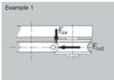
**Example 1 :** a roller is loaded with an axial force  $F_{ax} = 60$  N and a radial force of  $F_{rad} = 100$  N at a speed of 120 m/min.
