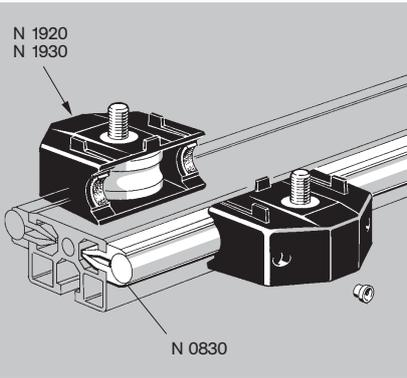
The linear guidance system K12 consists of steel guide rails hardened to 60 HRC fitted into the slot of NORCAN profiles and steel rollers on shielded (zz) bearings individually protected and lubricated by cassettes of PA compound. The lubricators allow to re-oil the felt-type scraping seals (don't use grease !).
