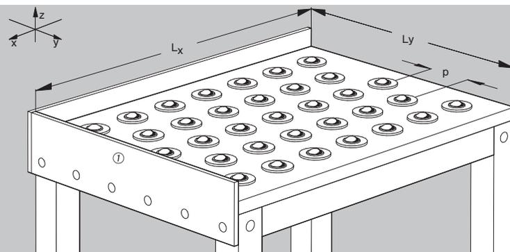
**Ball table** : for the transport of panels, flat bottom containers, cardboard packages, and other flat surfaced objects.
