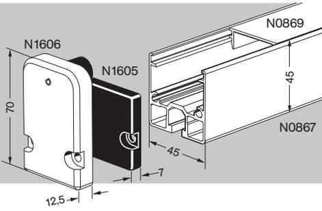
**U section profile 45x45 - N 0867** : for roller units. Material: anodised aluminium.  $I_y = 5 \cdot 10^4 \text{ mm}^4$
