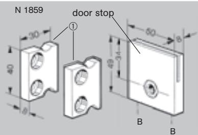
**Kit 2 for quick removal of panels - N 1859** : with screws and nuts. Same application as N 1860. The parts ① are prevented from rotation by two fixing screws and unlike N 1860 can be fitted without resting on another piece.
