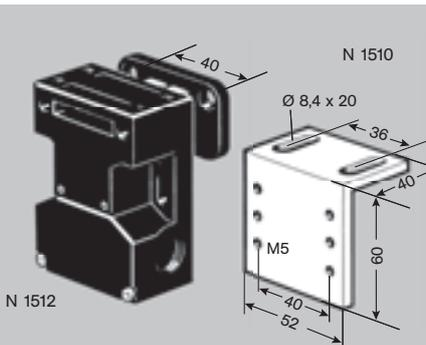
**Safety Switch Schmersal AZ 15 - ZVRK - 30N - N 1512** with nuts, screws (switch key entered = 1 contact closed). Retaining force 30 N.
