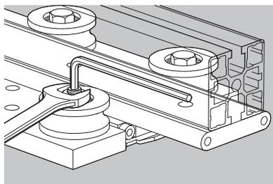
**Assembly :** First mount the rollers with eccentric shafts. Screw in that shaft completely whilst holding the nut with a #13 spanner. Then undo the shaft about a half turn into the position "maximum play". Tighten the nut very slightly. Mount and tighten the rollers with concentric shafts.
