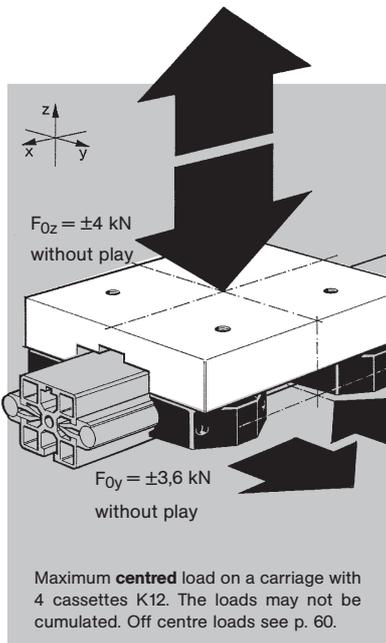
**Linear guidance system on cassettes with steel rollers K12** (p. 54): rigid guidance without play on hardened steel rails.
