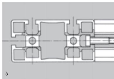
For applications where the standard assembly with the M8 x 43 through-bolt cannot be used.
