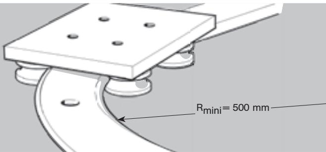
**Curved rails for guidances :** the rails for the linear guidance system NAP57 may be curved to a minimum radius of 500mm.
