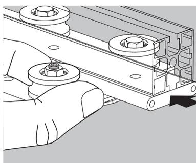
**Adjusting :** With a #13 flat spanner hold the nut of the roller with eccentric shaft and eliminate the play when turning the shaft with a #4 Allen wrench. Hold the Allen wrench in this position and firmly tighten the nut with the #13 flat spanner.
