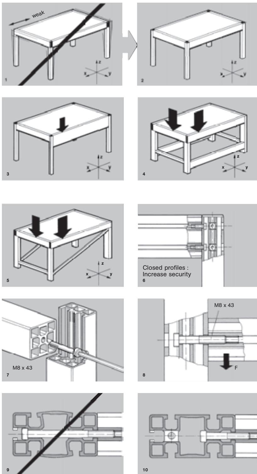
**Stiffness :** As a rule, a structure of given dimensions can be constructed with NORCAN profile in different design formats. The different designs do not provide the same stiffness or load bearing capabilities.
