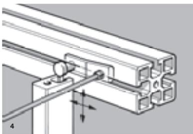
Fig. 4 and 5 show mountings with the adjustable coupling "X" - N 1148 and the assembly plates N 1110 or N 1111.
