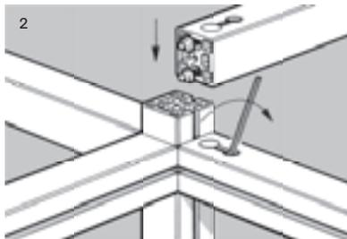
The example shows an assembly possible with M6 x 30 and M6 SC nut.
