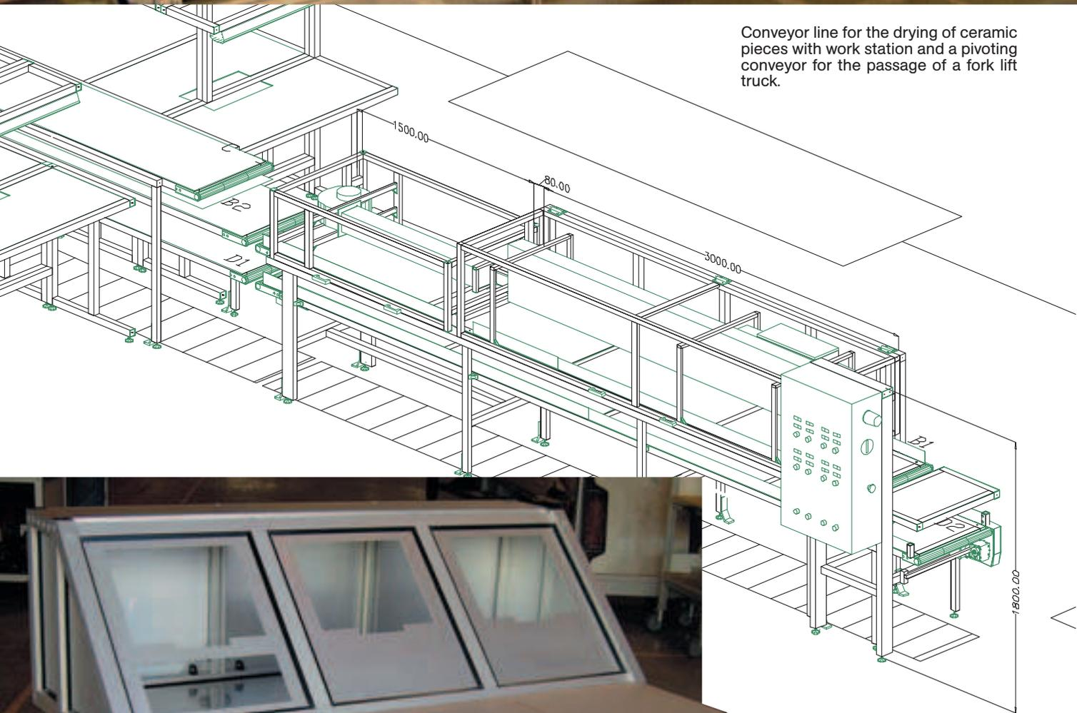
Conveyor line for the drying of ceramic pieces with work station and a pivoting conveyor for the passage of a fork lift truck.
