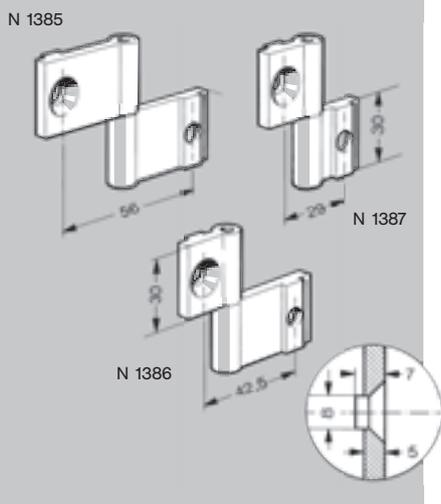
**Hinges, blind** with 2 M8 x 16 screws and M8 SC nuts : consist of two plates in aluminium and one zinc plated steel shaft. The hinges can face left or right and the shaft is locked when assembling.
