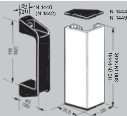
**Handle 116 CTRS - N 1440** with two M8 x 20 screws and two M8 SC nuts. Fits on 45 x 45 and 45 x 90 mm NORCAN profiles. Material : black polyamide. Width 25 mm, over all length 139 mm.
