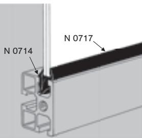
**Mounting profile - N 0717** allows assembly and disassembly of glass panels and other panels from 5 to 8 mm inside existing frames without dismantling the frames.
