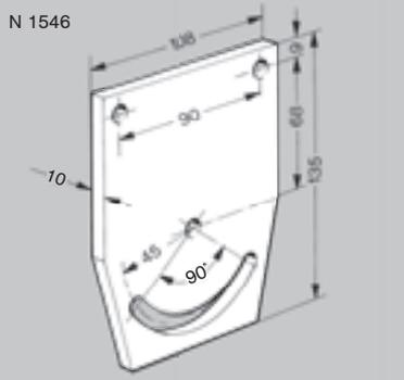
**Aluminium adjustable plate N 1546** with 3 M8 x 20 screws, M8 SC nuts and washers. For adjustable structures, accessories, conveyors etc.
