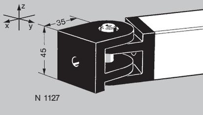
**Pivot 45 x 45, dynamic - N 1127** with 2 low head screws M8 x 20 mm. Fits on either the cut end or the side of the profile. For dynamic mountings from +90° to -90°. Maximum torque around the y-axis: 135 Nm (elastic limit). Material: aluminium alloy anodised black.
