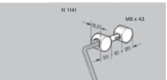
**Assembly nut, double - N 1141** with M8 x 43 screw for end-to-end fixing of profiles under low load
