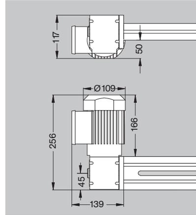
**Linear drive and guidance module PEV** : combination of a carriage on smooth guides N1363 (p.57) and a Tr 16x4 trapezoidal screw incorporated in a 45x90 NORCAN profile ( $T_{max} = 60^{\circ}C$ ).
