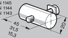
**Angled assembly coupling 45 long - N 1145** with M8 x 30 screw and square washer.
