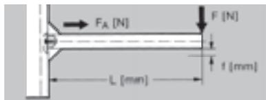
**Method B31 :** NORCAN 45 x 45 mm fixed with 1 central screw M8 x 20. plus 2 corner triangles
