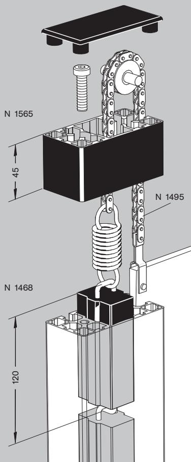
**Counterbalance with chain - N1565** : for vertical sliding panels. Consists of a length of 45x90mm NORCAN profile equipped with a pulley and 2m of 8mm chain with, on one side, a stainless steel fixing for 8mm panels or a guide profile N 1347 and, on the other side a spring for attaching up to 8 counterweights of 1kg N1468.
