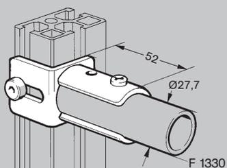
**Joint profile / tube ø27,7 open - F 1330** with screws and nuts: to mount ø27,7 CARENAL steel tubes on NORCAN - profiles. Allow a 4mm gap between the straight cut of the pipe and the profile. Material: Galvanised steel.
