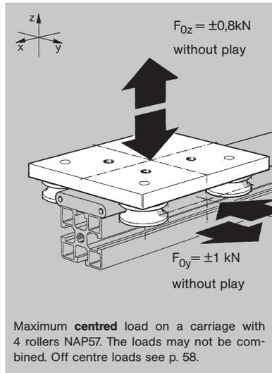
**Linear guidance systems on polyester rollers NAP57** (p. 52): guidance without play, smooth and silent in operation running on anodized aluminium rails.
