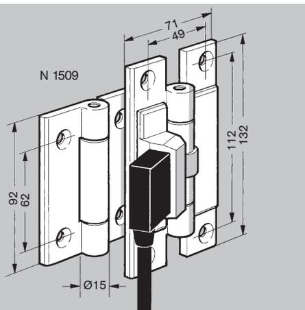
**Hinge kit with switch – N 1509** : comprising 1 hinge and 1 hinge with security switch, 8 screws M8 x 20 zinc plated and 8 nuts M8 SC. Compatible with th hinge 90/46 - N1507. Maximum opening angle 135°. Contact NO at 15°. Cable lenth 3m. Material: anodised aluminium alloy.
