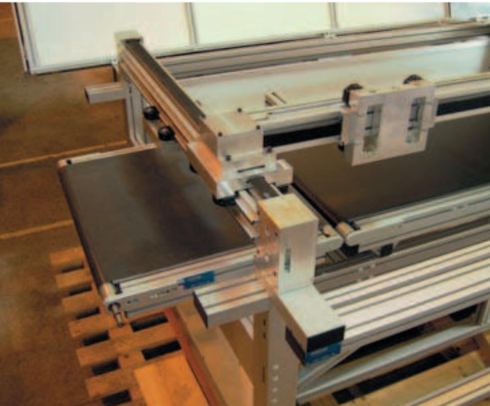
Machine frame with integrated guards, conveyors and an axis xy for very high accelerations.
