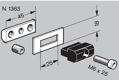
**Smooth guide - N 1363 :** For robust and particularly shock resistant linear guidance systems. Ideal for combinations with trapezoidal screw drives. For clearance free linear guides utilise the types "NAP 57" (p. 58), "K12" (p. 60) and "LF" (p. 63).
