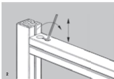
**Adjustable mountings :** Mountings with central bolt allow a limited adjustment only. For longer adjustments, we recommend :
