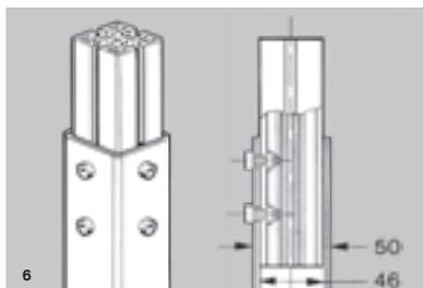
**Telescopic mountings :** standard 50/46 square tubing can be used for the construction of table legs, cantilevered mountings, and other telescopic or sliding mountings. The fixing is made with two pairs of nuts at 90° (do not position the screws across the axis of the profile - danger of deformation !) (fig. 6).
