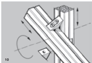
**Angled mounting** (fig. 9) : Profiles cut at an angle of 45° can be assembled directly using a M8 x 20 screw and a M8 SC nut. For all other angles use the angled assembly coupling N 1145.
