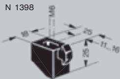
**Fixing block 1/4 turn - N 1398 :** for fixing 1..5 mm thick panels on the slotted sides of profiles N0163, N 0164, N0195, N 0264 and 1..19 mm panels on the slotted side of any other NORCAN profiles.
