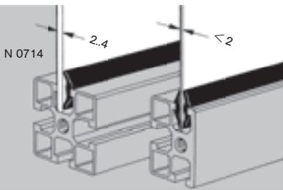
**Mounting strip - N 0714**, to hold plates and glasses 2 to 5 mm thick in position inside the slot (for plates under 2 mm use 2 strips!).
