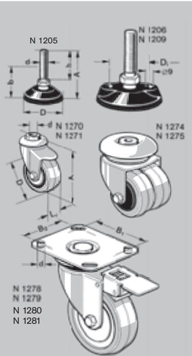
**Adjustables Feet :** black polyamide feet with antivibration pad and swivelling bolt. Refer to table underneath for types and dimensions.
