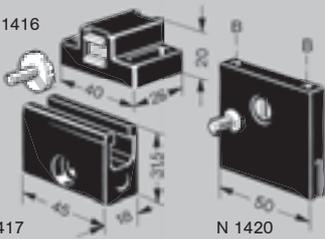
**Catch double sided magnet - N 1416 :** with 2 M6 screws and 2 M6 SC nuts. Receptacle with M5 stud and M5 SC nut. Magnetic force 15 and 30 N.
