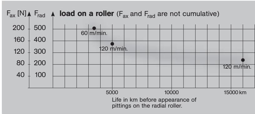
**Life and allowable loads :** The table opposite represents the results of a series of tests. These tests were undertaken without lubrication under a closed housing
