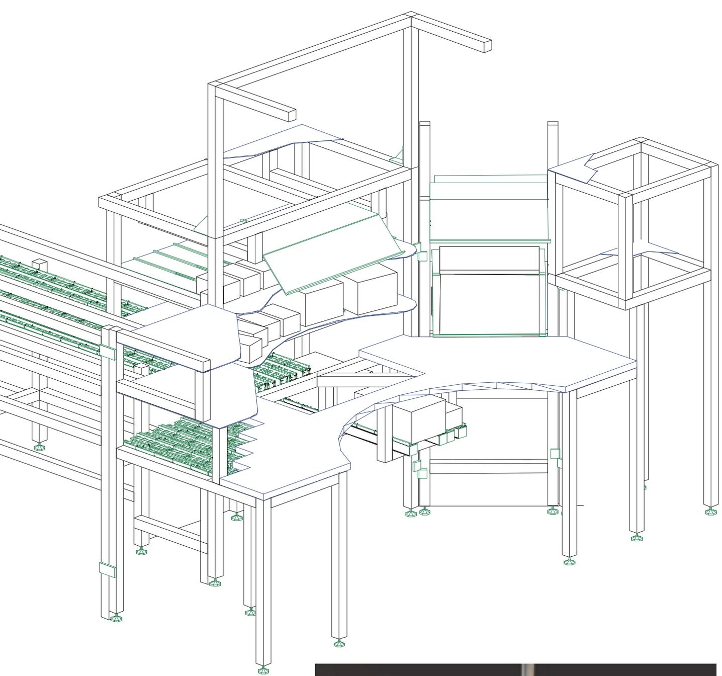
**Live storage** for workstations made from conveyor rails N0867, N0868 and guide rails N0804 (p.68/69) in several versions:
