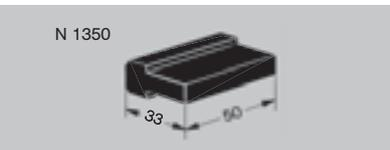
**Guide profile 1350** : For linear guides, must be locked with a screw through the profile.
