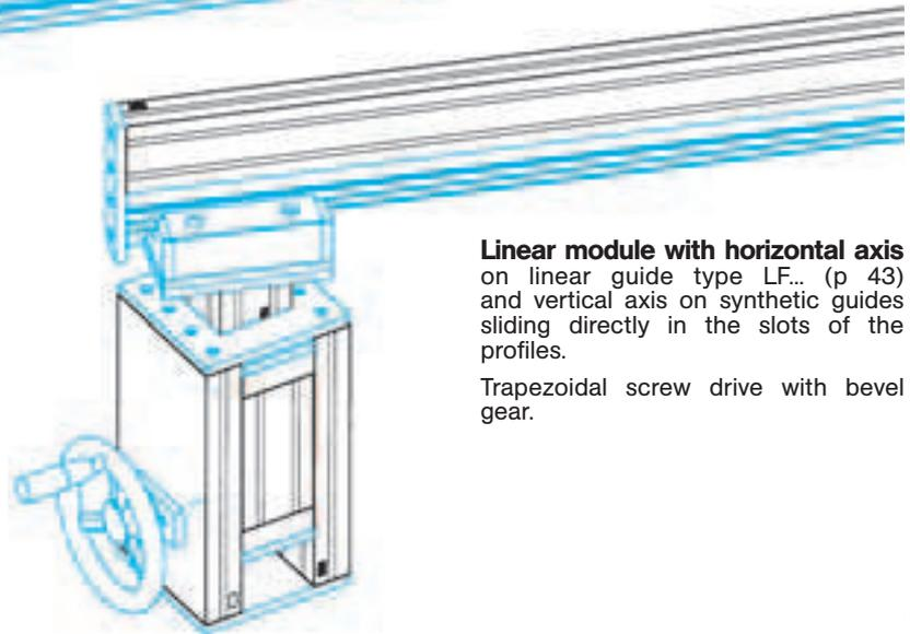
**Linear module with horizontal axis** on linear guide type LF... (p 43) and vertical axis on synthetic guides sliding directly in the slots of the profiles.
