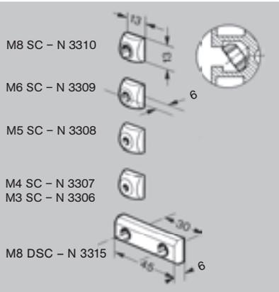
**Nut SC** zinc plated steel - can be tilted and inserted in the slot, thus permitting the attachment of various elements to existing structures without any need for dismantling. Plastic foam retainers N 3301 help to retain the inserted screw in position in vertical slots. Spring nuts ...RSC and ...RLSC see on bottom of this page.
