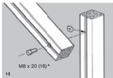
\*) Fig. 11, 12, 13 : M8 x 16 screw, when assembling without pressure washer and nut inside a profile slot of heavy profiles.
