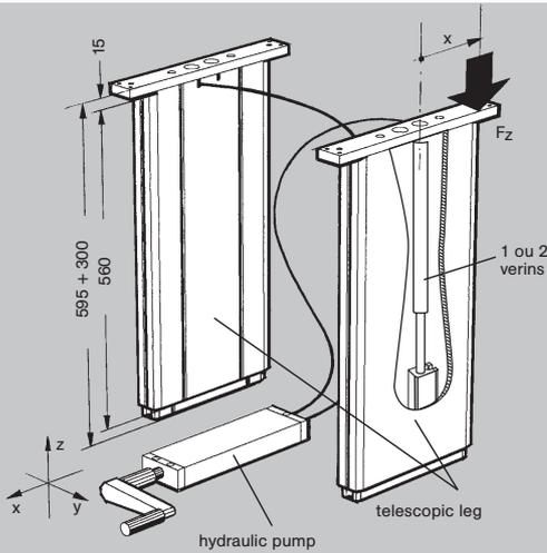
**Telescopic hydraulic legs** with 1 or 2 simple acting hydraulic cylinders per leg for height and angle adjustment of ergonomic workstations, bureau furniture, chariots, mobile frames, machines, conveyors etc.
