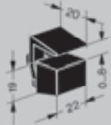
**Panel fixing block 1/4 turn - N 1399 :** for 1...8 mm thick panels on the slotted profile side. Assembly without tools, dismantling with a small screw-driver or similar.
