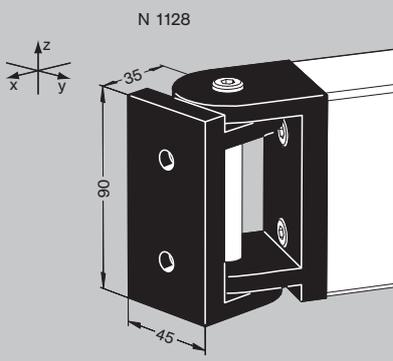
**Pivot 45x90, dynamic - N 1128** : with 2 low head screws M8 x 20. Fits on either the cut end or the side of the profile. For dynamic angle mountings from + 90° to - 90°.
