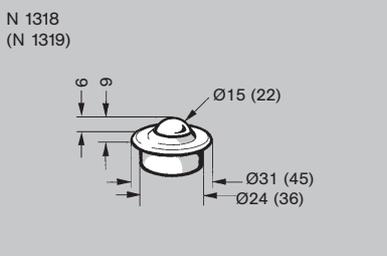
**Ball caster  $\varnothing 15$  bushing  $\varnothing 24$  - N1318**
