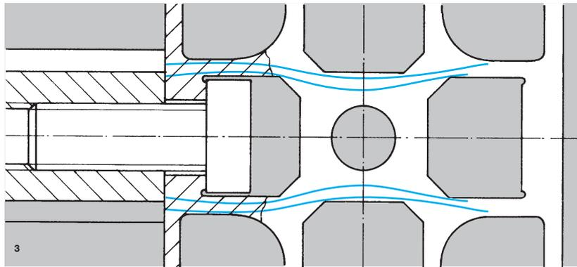
**2.** The NORCAN profiles have a deep slot allowing a large end play of the screwheads and nuts (figs. 4 and 5).
