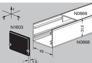
**U section profile 31,5 x 45 - N 0868** : light profile for roller units. To be mounted with screws or double sided adhesive tape onto NORCAN structures. Material: anodised aluminium. I<sub>y</sub> = 2 · 10<sup>4</sup> mm<sup>4</sup>
