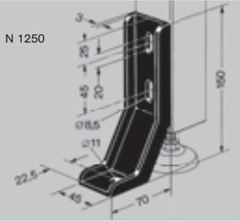
**Anchor Angle - N 1250** : with 2 M8 x 16 screws, 2 washers and 2 M8 SC nuts : used to anchor the uprights of structures on the floor.
