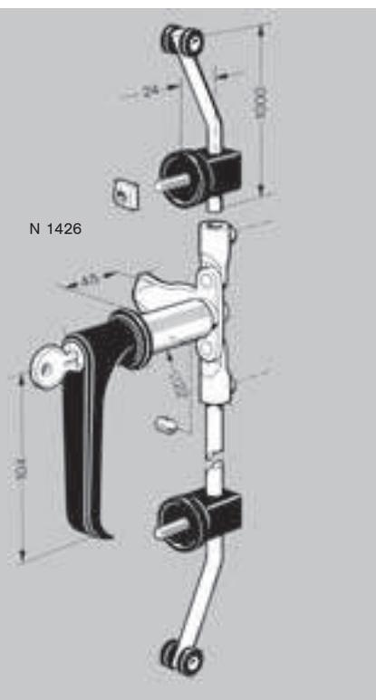
**Locking handle with rod - N 1426** :  $\varnothing$  22 mm, for 18, 31,5, and 45 mm thick doors. The rods are 1000 mm long and have to be cut to suit.
