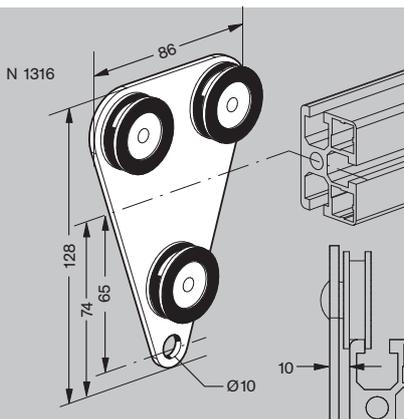
**Tool support on 3 rollers - N1316**: low friction, for NORCAN - Profile 18x45 N0162 and 31,5x45 N0164. Maximum load 10kg, avoid lateral loads
