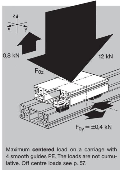
**Smooth guides PE** (p. 51): economical and robust linear guidance, particularly shock resistant in the -z direction (3kN). Ideal for combinations with trapezoidal screw drives.
