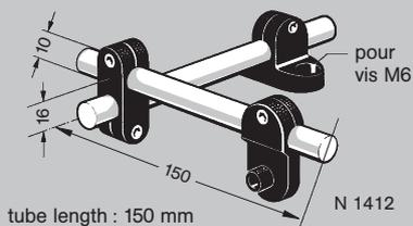
**Sensor-support - N 1412 :** adjustable support for photocells, limit-switches and other types of switches with a diameter of 19 mm used for automation.
