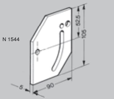
**Plate, footrest, adjustable N 1544** with 3 M8 x 20 screws, 2 M8 SC nuts 3, washers and 1 locking finger. The profile "A" can be adjusted from 0° and 45°.
