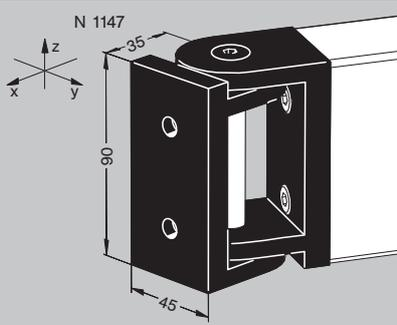
**Pivot 45X90 - N1147** with 2 low head screws M8 x 20. Fits on either the cut end or the side of the profile. For fixed angle mountings from +90° to -90°.
