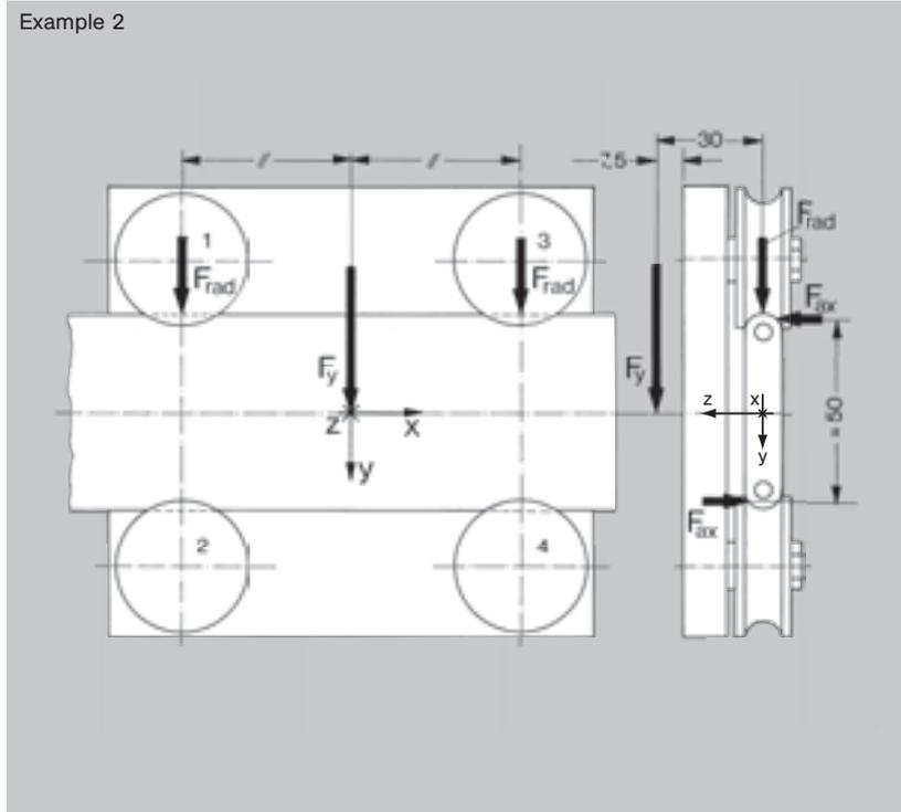
**Example 2 :** For the carriage opposite there is a static force,  $F_y = 240$  N acting on a point 7,5 mm above the centre of the carriage,  $v = 2$  m/s.
