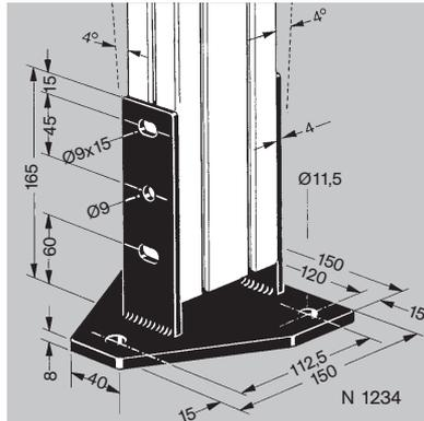
**Anchor foot - adjustable 45 - 3 points - N1224:** with 6 M8 x 20 screws, 6 washers and 6 M8SC nuts. Used to anchor uprights made of 45mm profiles to the floor.
