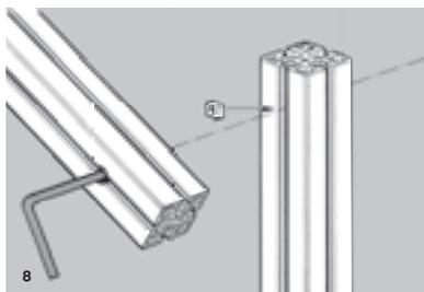
**Orientable mountings :** Assemblies with nuts and bolts allow the construction of orientable structures. With a fixed rotation axis, use a SC nut and a M8 x 43 screw (fig. 8). With a sliding rotational axis the assembly with 2 or 4 corner triangles (fig. 10) or with the adjustable coupling "X" (fig. 4) will give a possibility of movement in 2 directions.
