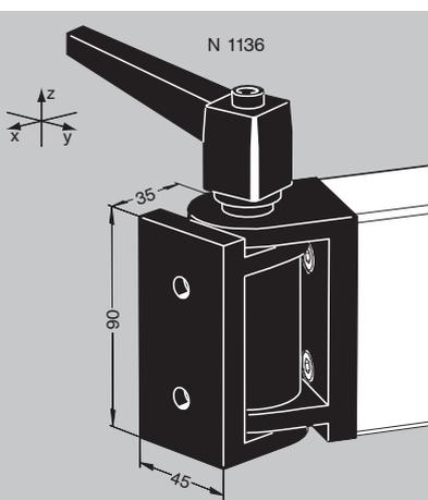
**Pivot 45x90 with locking handle - N 1136** : with 2 low had screws M8 x 20. Fits on either the cut end or the side of the profile. For angle mountings from + 90° to - 90°. Tightening the handle with 20 Nm will lock the pivot with about 45 Nm.
