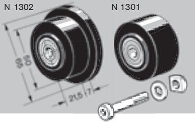
**Shouldered Linear Guide Roller - N 1302** : Roller in PA 6.6 on two bearings and secured by central bolt M8.
