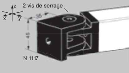
**Pivot 45 x 45 - N 1117** with 2 low head screws M8 x 20 mm. Fits on either the cut end or the side of the profile. For fixed angle mountings from +90° to -90°. Maximum torque around the y-axis: 135 Nm (elastic limit). Material: aluminium alloy anodised black.
