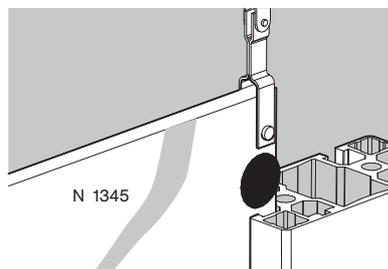
To avoid the crabbing or jamming of sliding panels, especially if the ratio of height to width is smaller than 0,7 the panel should be equipped with ball bearings N1315 or pads for sliding doors N1345 to assure a smooth linear guidance.
