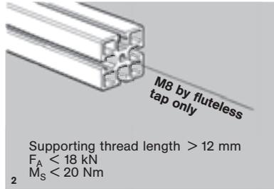
The figures 2-11 opposite illustrate the main means of fixing M8 screws and nuts to NORCAN profiles.
