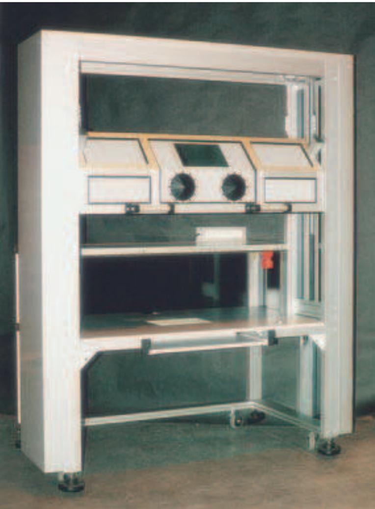
**Glove box** vertically sliding on roller guides with counterweights.
