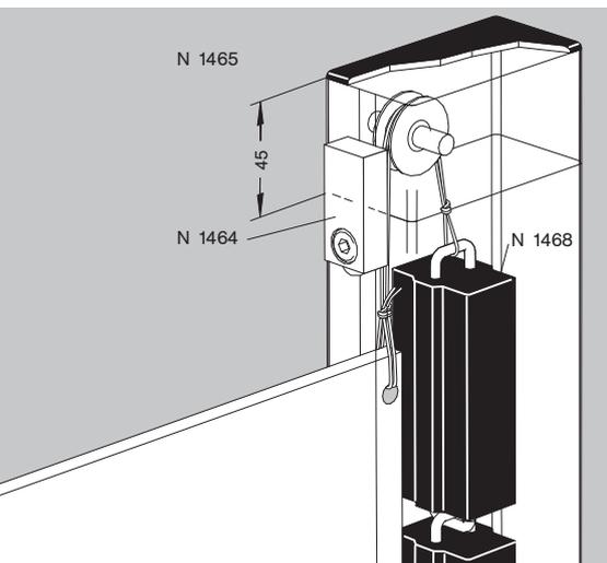
**Counterbalance for vertical sliding panels :** consists of a length of 45 x 90mm NORCAN profile equipped with a pulley and suspended counterweight. For low cost construction or sliding doors made of polycarbonate 8 mm thick.
