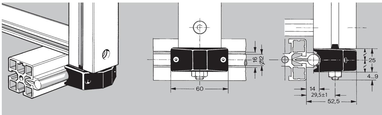
Direct mountings of K12-cassettes onto NORCAN profiles and plates. Indirect mounting with strut profile see below
