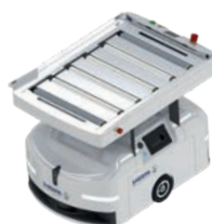
Front conveyor (bin 800x600 mm)
